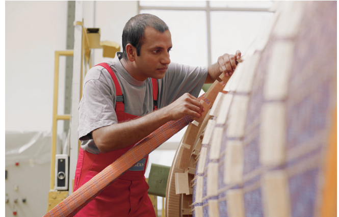
Windings made of transposed conductors reduce additional losses to a minimum
