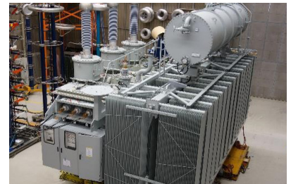
Transformer 100 MVA, single-phase 60 Hz Resilience transformer
