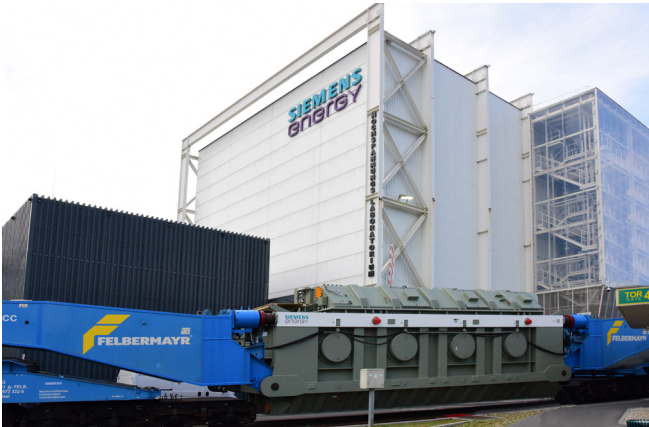
Transport of a transformer tank
