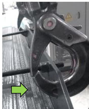
Image 5-5: Crane hook with distance to upper yoke
