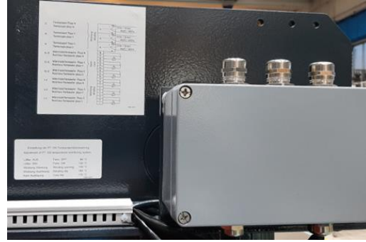
Image 6-15: Power connector for fan (Example)
