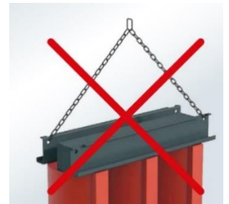
Image 5-3: NOT correct lifting of the transformer
