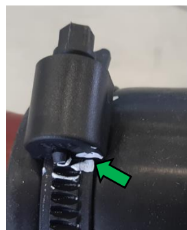
Image 8-3: Position of the color marking on the clam after tightening
