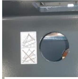
Image 5-1: Marking lifting lugs for crane hooks
