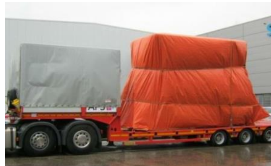
Image 5-8: Lashing the transformer to the loading area
