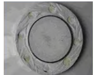
Horizontal cut of a cage design arrester
