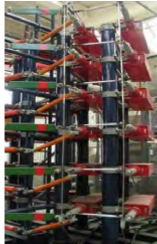
Test generator supplying both impulse voltages (1.2/50 \mu s and 250/250 \mu s) and impulse currents (8/20 \mu s and 30/60 \mu s)
