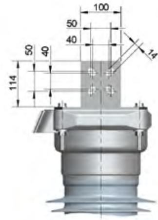
DIN/NEMA flat terminal 3EQ4 ...-.....-R.. (copper) 3EQ4 ...-.....-T.. (aluminum) 3EQ4 ...-.....-X.. (hot dip galvanized) 3EQ4 ...-.....-Y.. (stainless steel)
