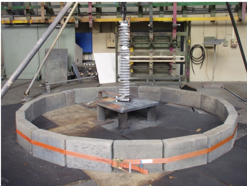
Figure 25: Polymer-housed arrester ("cage-design") after a short-circuit test at rated current (65 kA, 200 ms). The housing is ripped but in mechanically sound condition. Details of the test setup can well be seen. For further information see short-circuit tests in the appendix.
