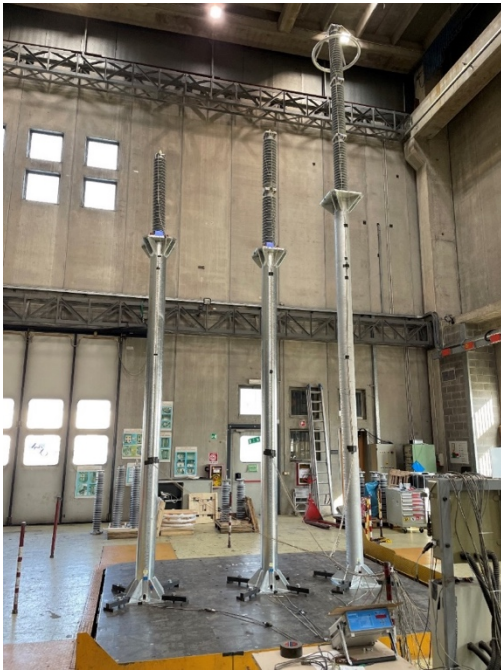
Figure 24: Polymer housed arresters for system voltages of U_s=170 kV, U_s=245 kV and U_s=420 kV during seismic testing on a shaking table
